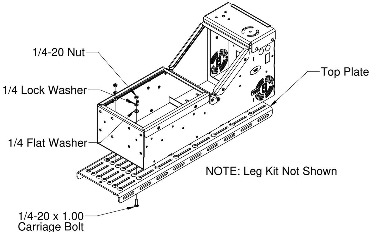
**FIG 1 - Console Installation on Top Plate**
