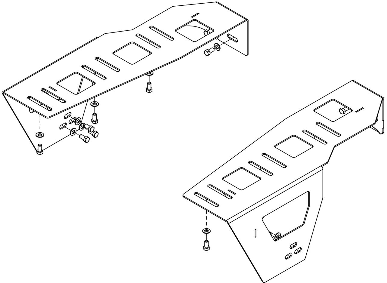
1. Remove three 3/8 hardware attached to each kicker rod lower on driver and passenger side.
