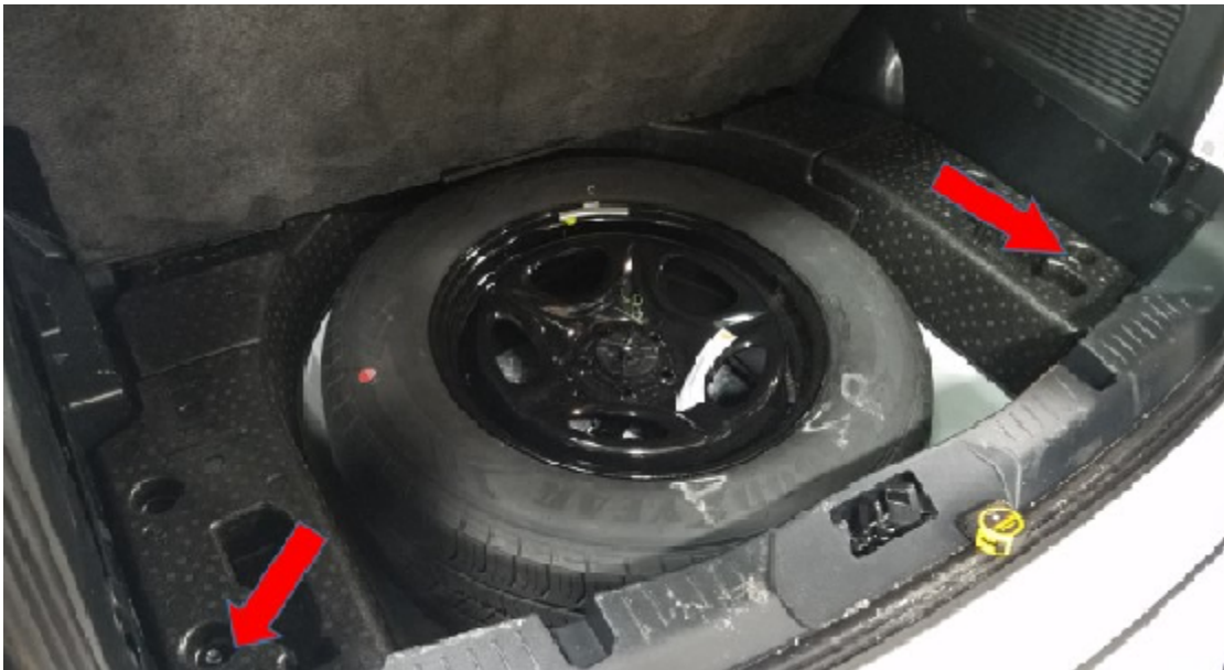
IMAGE FROM REAR END - 8MM BOLTS EXPOSED
