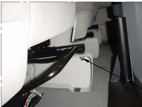
Move the front passenger seat rearward to gain access to the front inboard and outboard bolts. Remove the nuts from the bolts. Place an open ended wrench between the seatrail and seatbase onto the jam nut. Unscrew bolts using torx bit until you are able to lift seat enough to slide item 7160-0116 between the seatrail and seatbase. Retighten bolts back down and replace the nuts.
