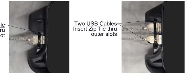
One USB Cable Insert Zip Tie thru center slot
