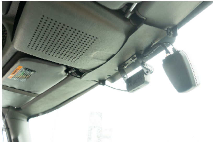
headliner mount with Samsara camera attached
