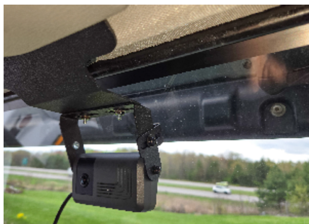
headliner mount with Samsara camera attached
