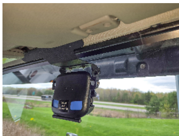
headliner mount with Lytx camera attached
