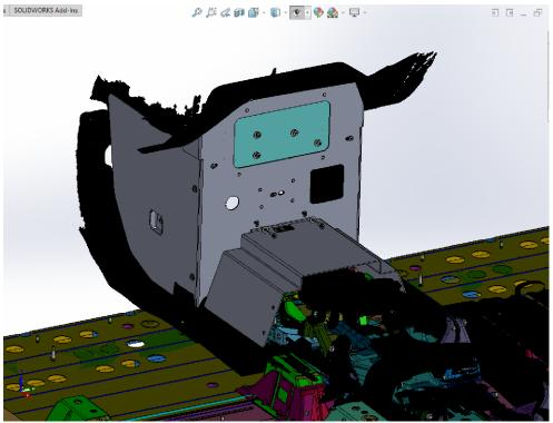
18. loosely attach the driver and passenger side leg brackets with the bolts
