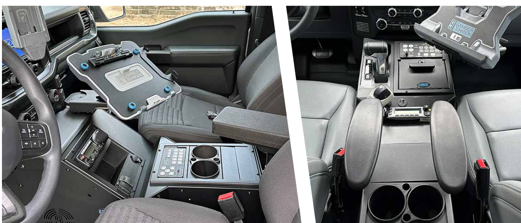
7170-1063-02 Wide Body Console Box with Internal Printer Mount, Cup Holder, Tall Rear Armrest and Mongoose® XLE 9" Motion Attachment
