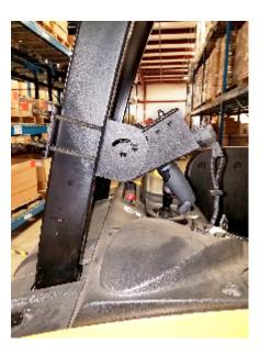
lock nuts to adjust width
